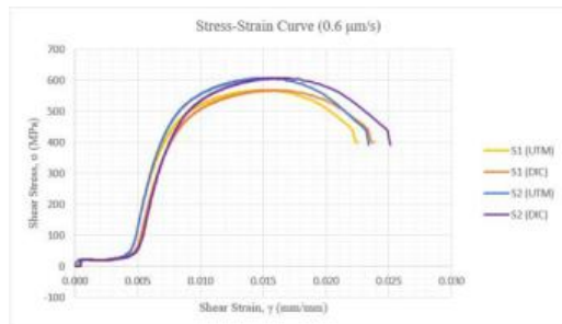
Fig. 3: Shear stress-strain curve plotted from data analysed at 0.6 \mu\text{m/s} grip displacement rate
