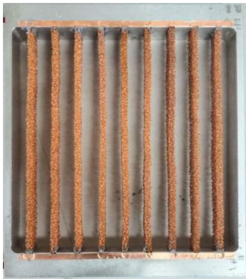
Fig. 2.1: Heat exchangers setup. (20 PPI, 15 mm spacing)
