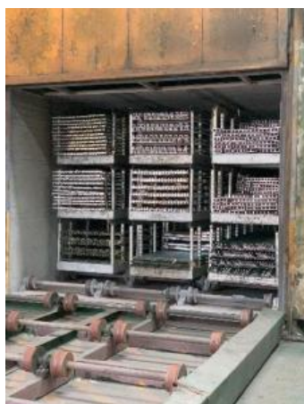
Figure 1 : The Position of alloys on the trolley inside the ageing oven
