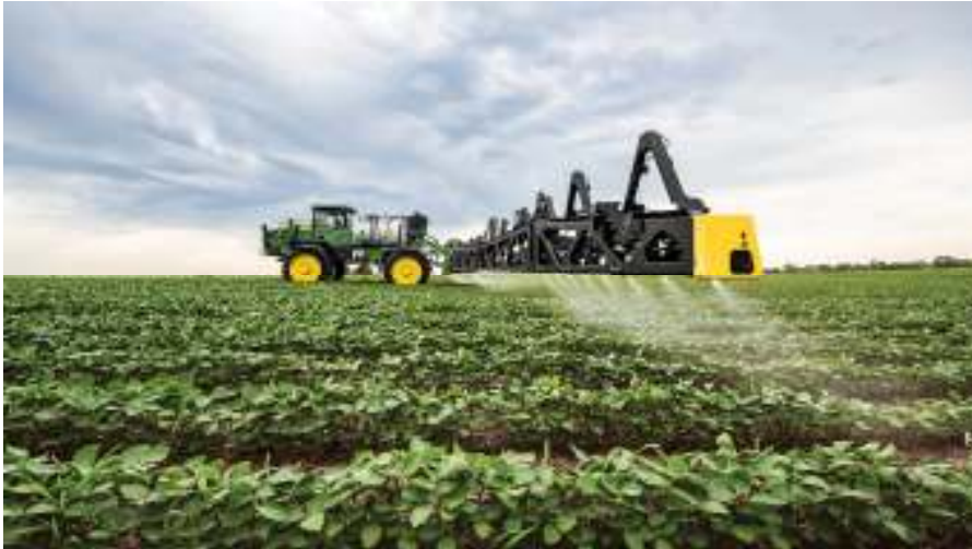
Blue River Technology's See & Spray robotic weeder uses computer vision to detect and spray individual weeds in cotton fields. Source: John Deere
